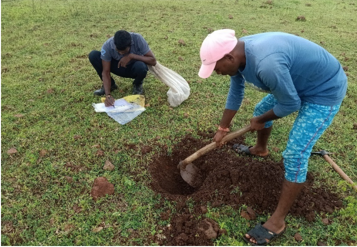
Field Photograph11: Pit being excavated to collect soil samples
