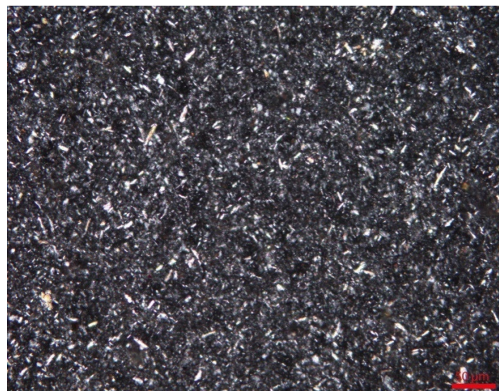
Pmg – 2: Photomicrograph showing very fine flaky aggregates of clay minerals as seen under crossed nicols.
