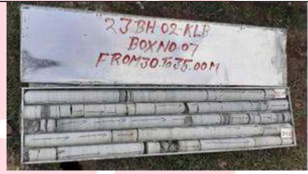
Figure 25: Light grey coloured, fine grained, hard, and massive limestone with thin intercalations of shale noticed. KALB 23BH02(G3).
