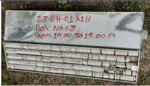
Figure 22: Cream coloured, fine grained, hard, and massive limestone. KALB 23BH01(G3).
