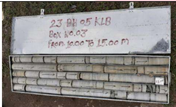
Figure 30: Light grey to cream coloured, fine grained, hard, and massive limestone with thin intercalations of shale. KALB 23BH05(G3).
