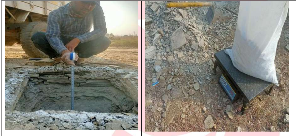
Figure 44: In situ bulk density test photos
