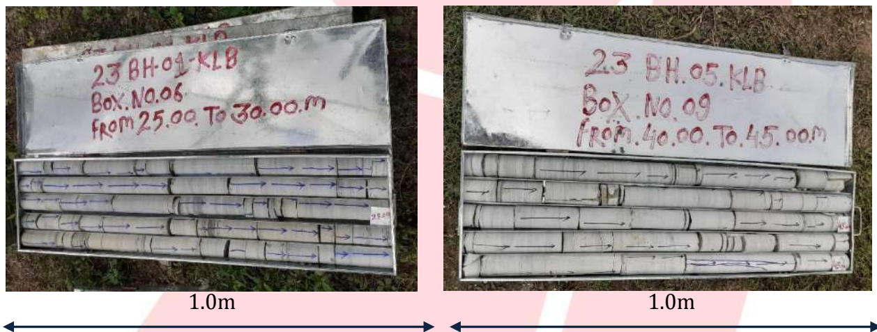
Figure 21: Drill cores of borehole KALB 23BH-01 and KALB 23BH-05 stored in G.I. Core boxes and the drilled cores kept in book pattern style
