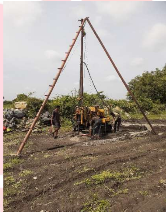
Figure 18: Hydrostatic diamond core drilling rig installed in borehole KALB 23BH-01 exploration block.
