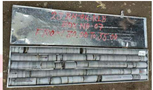
Figure 29: Light grey coloured, fine grained, hard, and massive limestone with thin intercalations of shale noticed. KALB 23BH04(G3).
