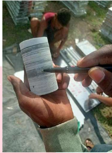
Figure 20: Detailed lithological core logging in borehole KALB 23BH-01 at site.
