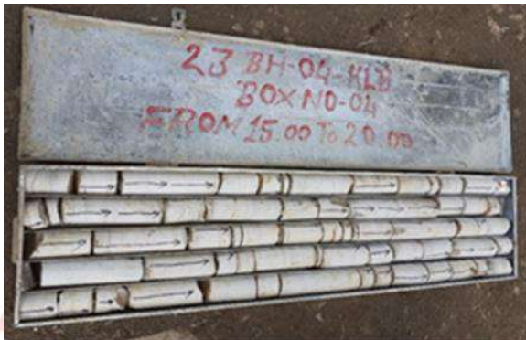
Figure 28: Cream to light gray coloured, fine grained, hard, and massive limestone. KALB 23BH04(G2).
