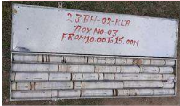
Figure 24: Cream coloured, fine grained, hard, and massive limestone. KALB 23BH02(G3).
