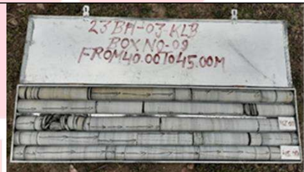
Figure 27: Light grey coloured, fine grained, hard, and massive limestone with thin intercalations of shale noticed. KALB 23BH03(G3).
