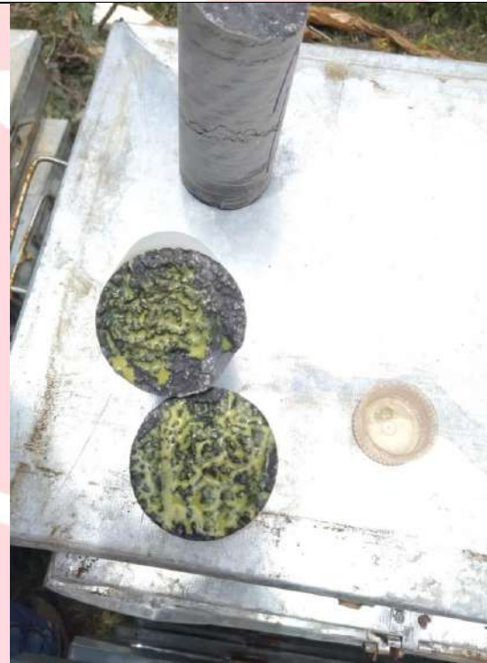
Figure 33: Shapiro's kit test showing positive result on drill core sample.
