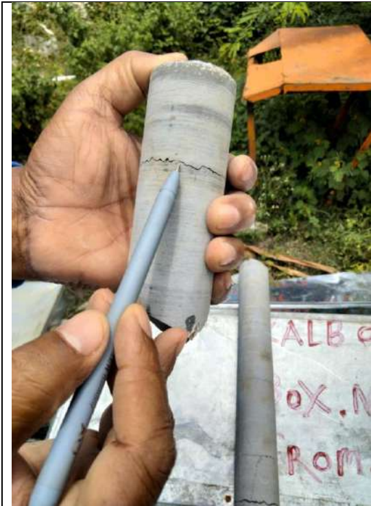
Figure 32: Thin band of Phosphorite observed in the drill core samples
