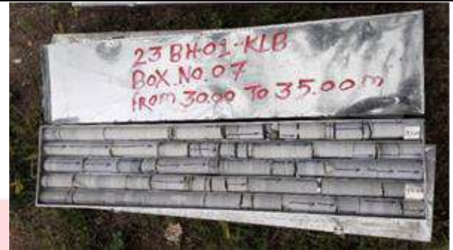
Figure 23: Light grey coloured, fine grained, hard, and massive limestone with thin intercalations of shale noticed. KALB 23BH01(G3).
