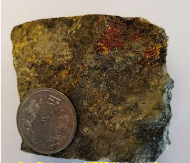
Core Photograph of MTCB-11 showing Copper mineralisation in Qtz-Bio Rock (Depth: 54.20-54.25m)
