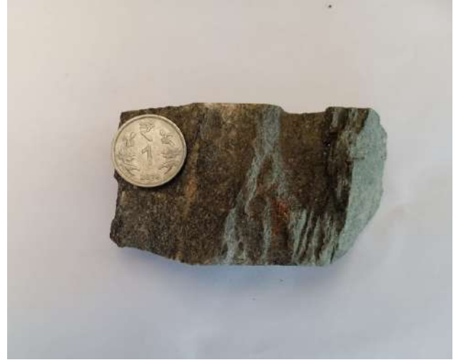
Photograph No.12: Core Photograph of MTCB-11 showing Copper mineralisation in Qtz-Biotite Rock (Depth: 54.20-54.25m)
