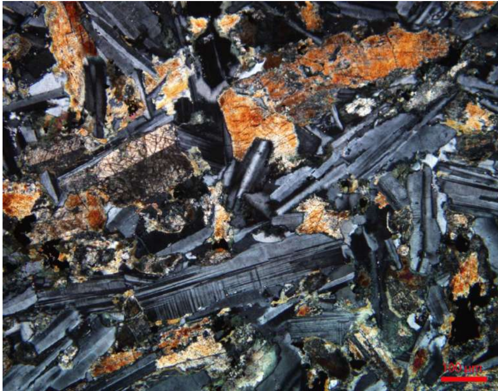
Pmg – 3: Photomicrograph showing sub-ophitic and inter-granular texture in dolerite as seen under crossed nicols.
