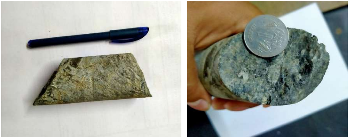
Photograph No.4: Core Photograph of MTCB-01 showing sheared Quartz biotite rock (Depth: 70.00 - 70.10 m)
