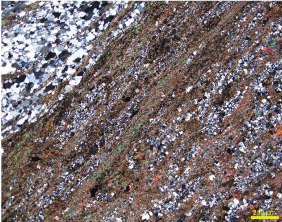
Pmg – 1: Photomicrograph showing association and parallel alignment of phlogopite and quartz, where phlogopite is seen segregating into moderately thick zones as seen under crossed nicols. Specimen No. : MTCB01/ P2 Magnification :40X
