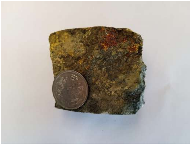
Photograph No.12: Core Photograph of MTCB-11 showing Copper mineralisation in Qtz-Biotite Rock (Depth: 54.20-54.25m)
