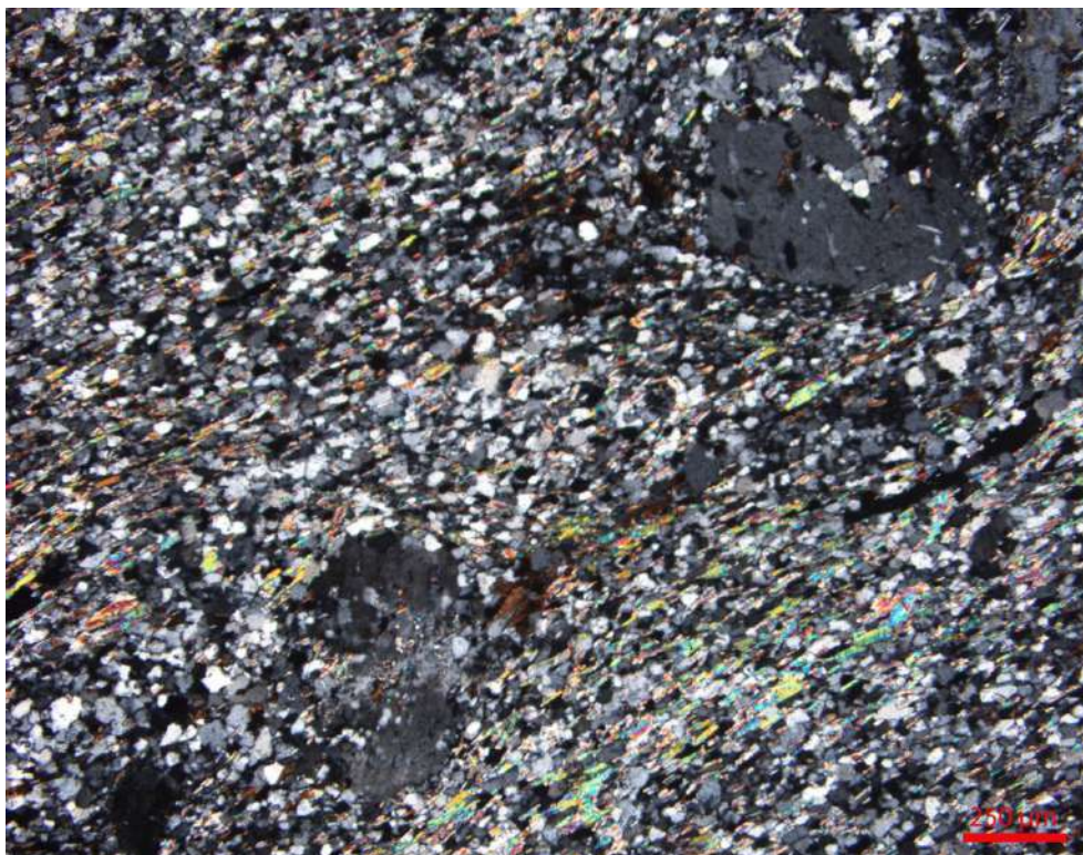
Pmg – 4: Photomicrograph showing association and parallel alignment of quartz, muscovite and albite, where albite is also seen present as medium to moderately coarse porphyroblasts with rotation as seen under crossed nicols.
