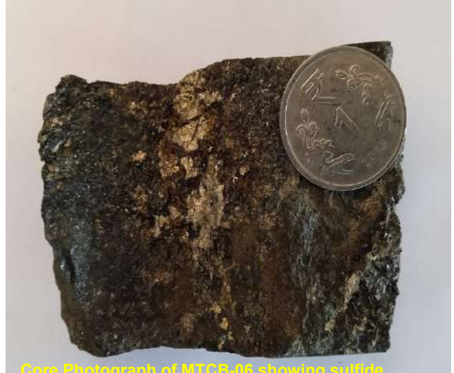
Core Photograph of MTCB-06 showing sulfide mineralisation in Chl-Bio-schist (Depth: 35.40-35.50m)
