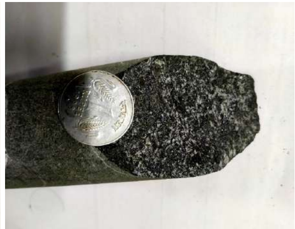
Photograph No.8: Core Photograph of MTCB-06 showing Amphibolite (Depth: 53.36m - 53.46m)
