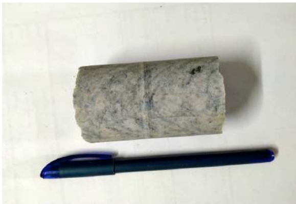
Photograph No.9: Core Photograph of MTCB-06 showing Granite gneiss (Depth: 94.54m - 94.62m)
