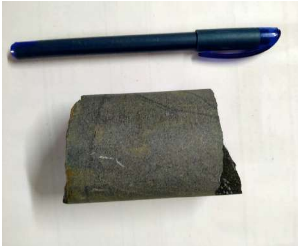
Photograph No.7: Core photograph of MTCB-06 showing Dolerite (Depth: 16.96m - 17.04m)
