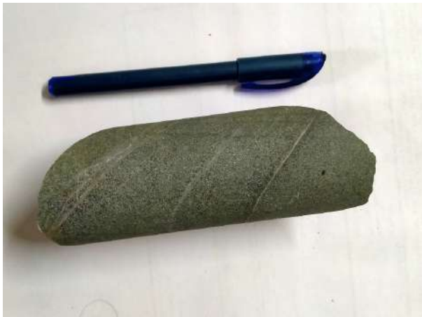
Photograph No.8: Core Photograph of MTCB-06 showing Amphibolite (Depth: 53.36m - 53.46m)
