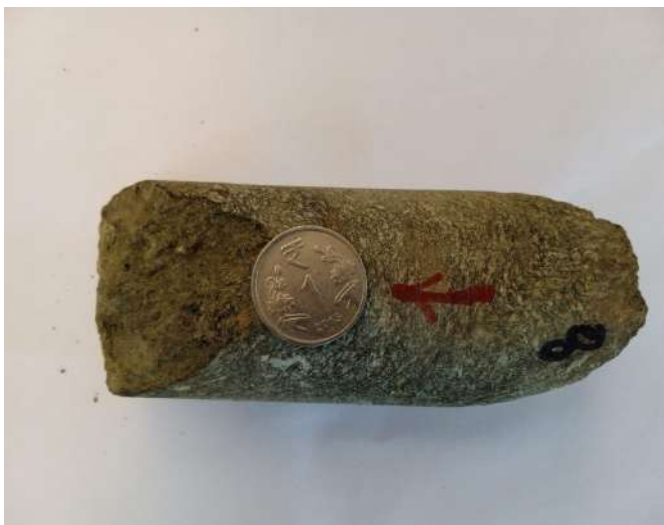
Photograph No.13: Core Photograph of MTCB-04 showing Granite gneiss (Depth: 82.0m-82.07m)
