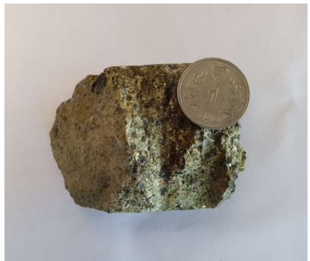
Photograph No.13: Core Photograph of MTCB-04 showing Granite gneiss (Depth: 82.0m-82.07m)
