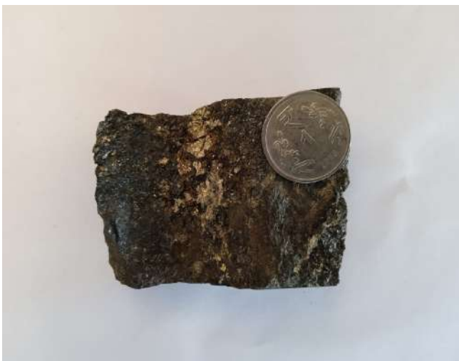
Photograph No.15: Core Photograph of MTCB-09 showing sulphide mineralisation in Biotite-schist (Depth: 76.10m -76.19m)
