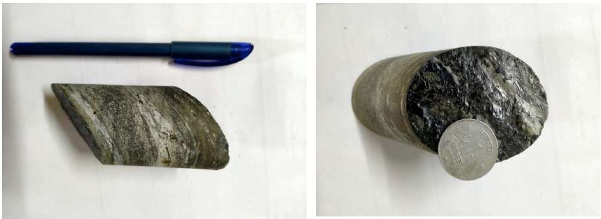
Photograph No.5: Core Photograph of MTCB-01 showing Chlorite biotite schist (Depth: 82.10 - 82.17m)
