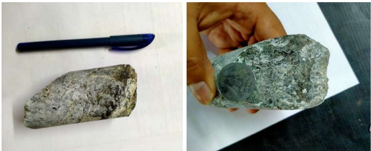
Photograph No.6: Core Photograph of MTCB-02 showing Granite (Depth: 39.90 - 39.99m)
