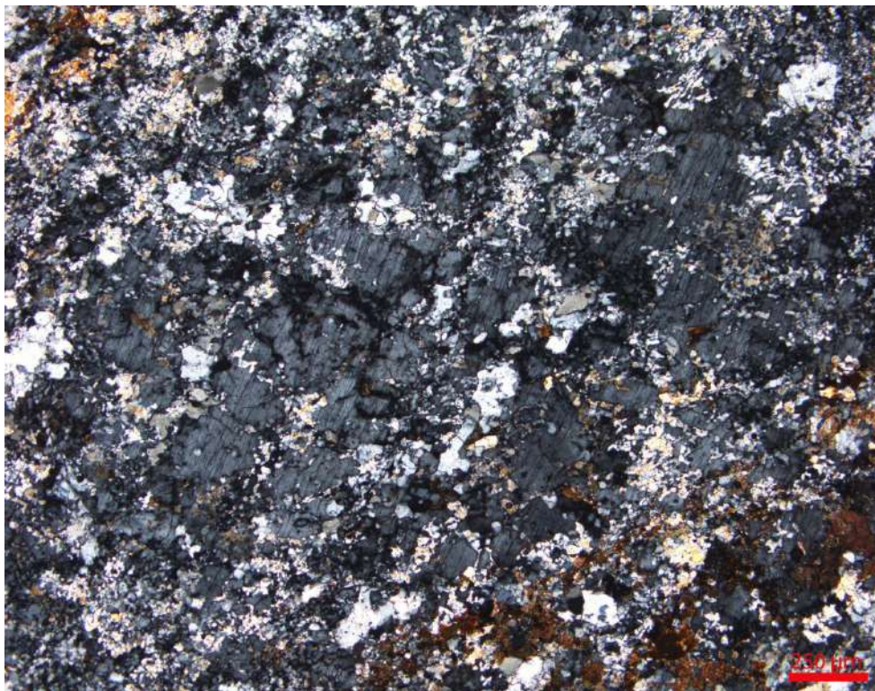
Pmg – 2: Photomicrograph showing albitization in biotite rich feldspathic (albitised) quartzite as seen under crossed nicols. Specimen No. : MTCB02/ P3 Magnification :40X
