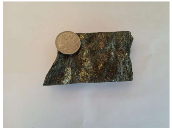
Photograph No.15: Core Photograph of MTCB-09 showing sulphide mineralisation in Biotite-schist (Depth: 76.10m -76.19m)
