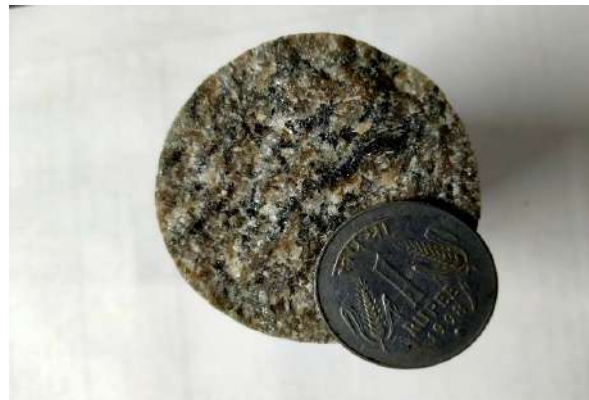
Photograph No.9: Core Photograph of MTCB-06 showing Granite gneiss (Depth: 94.54m - 94.62m)
