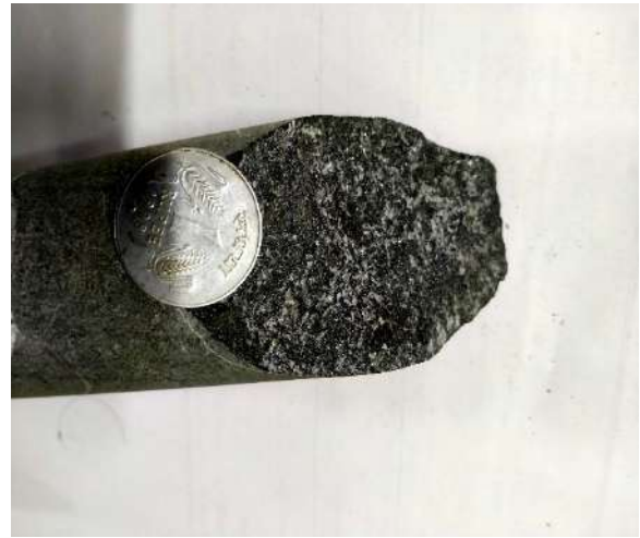
Photograph No.7: Core photograph of MTCB-06 showing Dolerite (Depth: 16.96m - 17.04m)
