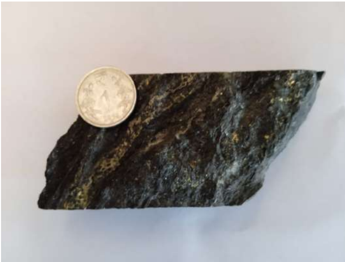
Photograph No.14: Core Photograph of MTCB-06 showing sulfide mineralisation in Chlorite-Biotite-schist (Depth: 35.40-35.50m)
