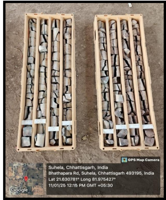
Photo. – 8.7: Half Splitted Core Of Borehole ALD-1
