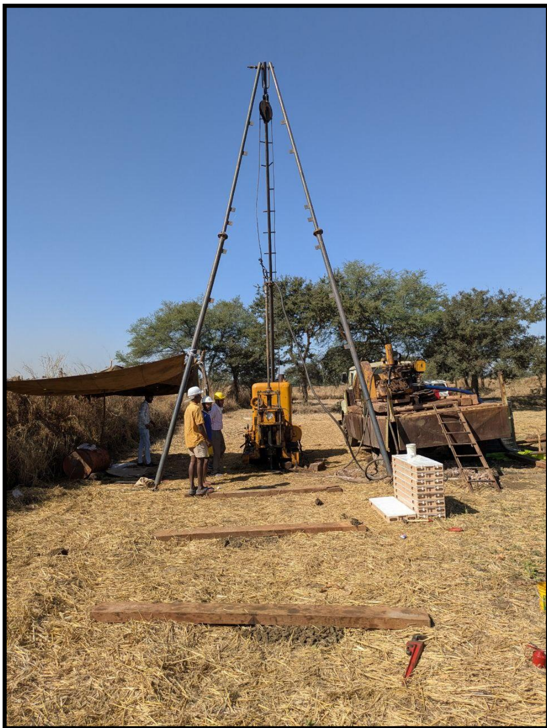
Photo-8.1 Drilling Operation By Drill No.06/Voltas 180 At BH No. ALD-12
