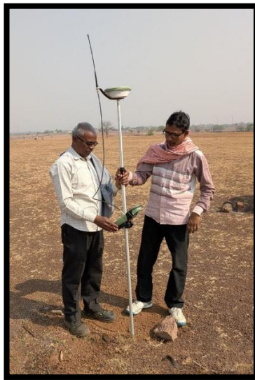
Photo-8.2: DGPS SURVEY (Make-Leica GNSS System, Model- Cs10)
