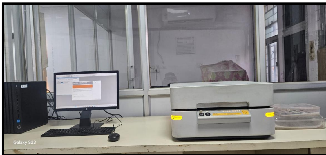
Photo -8.10: Photograph Of ED-XRF Instrument At Departmental Central Lab DGM, RAIPUR.
