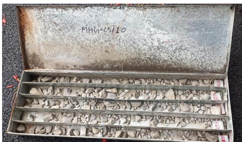
Photo- 6d: Core photograph showing dolomite zone (highly fractured) from 45.00m to 50.00m in Bh. No. MHG-05.
