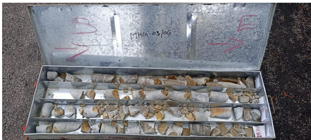
Photo- 6c: Core photograph showing dolomite zone from 24.00m to 28.00m in Bh. No. MHG-03
