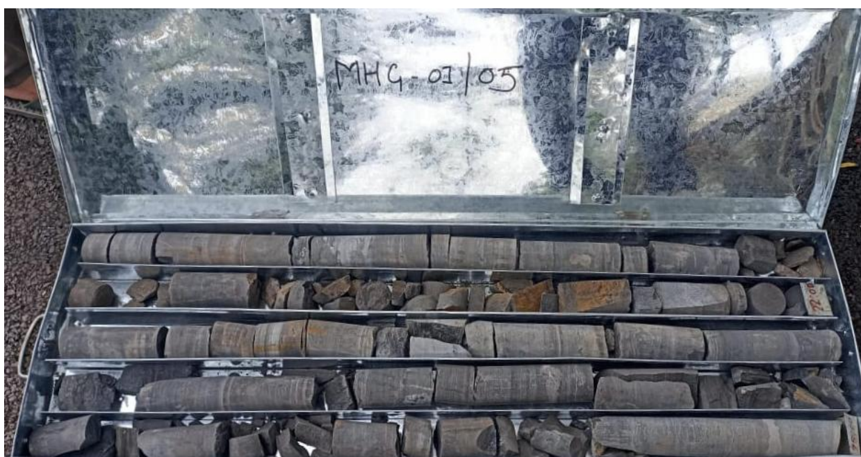
Photo - 02: Core photograph showing shale with calcite veins from 21.00m to 25.00m in Borehole No. MHG-01.
