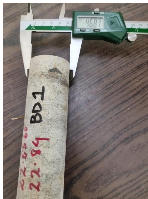
Photo 10: Photographs of dolomite core samples showing determination of length, diameter and weight of sample number HG/BD/01 for bulk density calculation.
