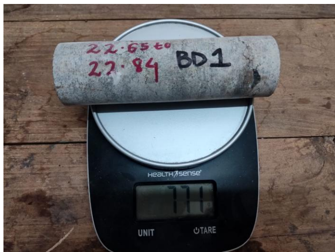
Photo 10: Photographs of dolomite core samples showing determination of length, diameter and weight of sample number HG/BD/01 for bulk density calculation.
