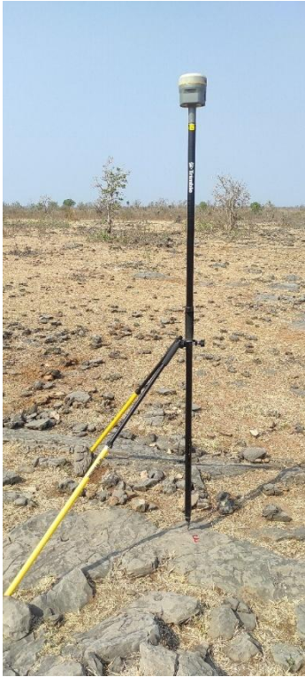
Photo 07: Photograph showing fixing of Block Boundary point through DGPS.
