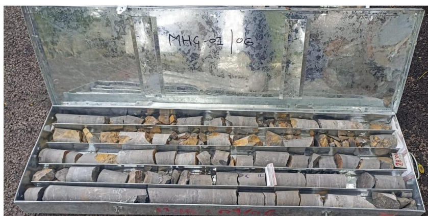
Photo- 6a: Core photograph showing dolomite zone from 25.00m to 28.50m in Bh. No. MHG-01
