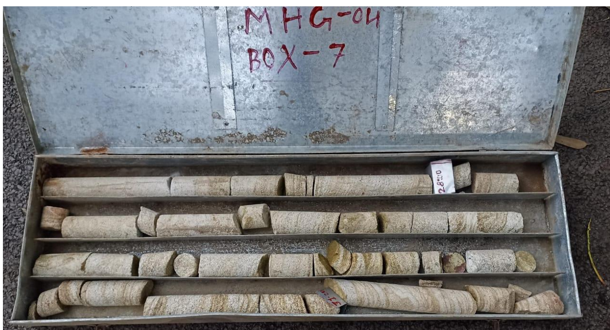
Photo - 01: Core photograph showing sandstone from 27.40m to 31.60m in Borehole No. MHG-04.
