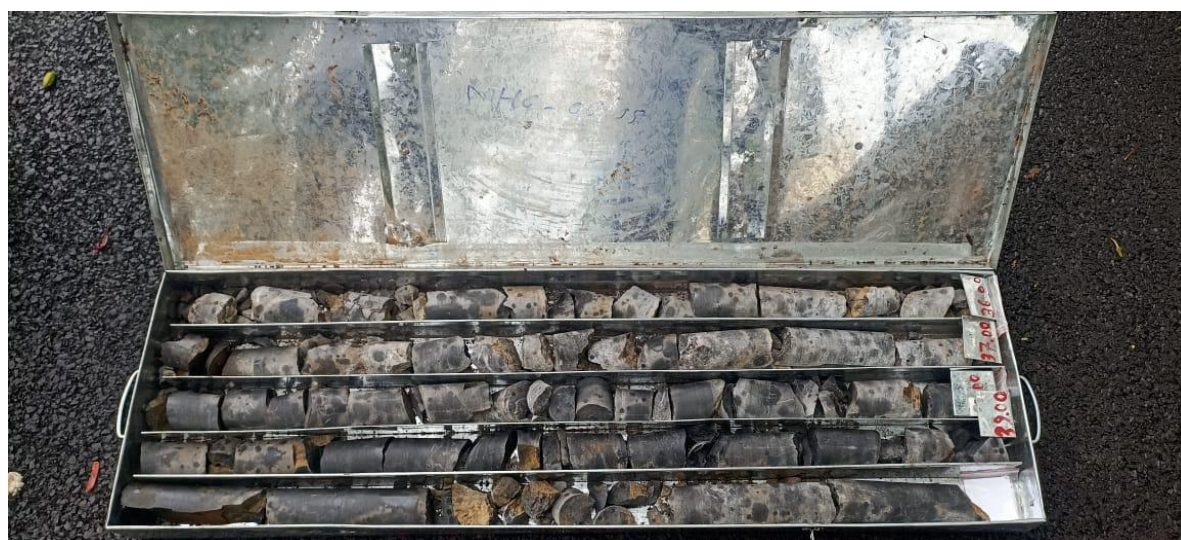
Photo- 6e: Core photograph showing dolomite zone from 35.00m to 40.00m in Bh. No. MHG-06.
