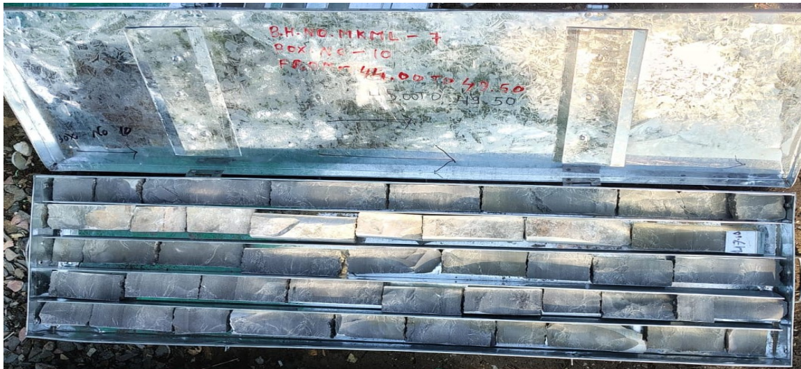
Photo - 10: MKML-09 (45.00-50.00) HALF CUT CORE
