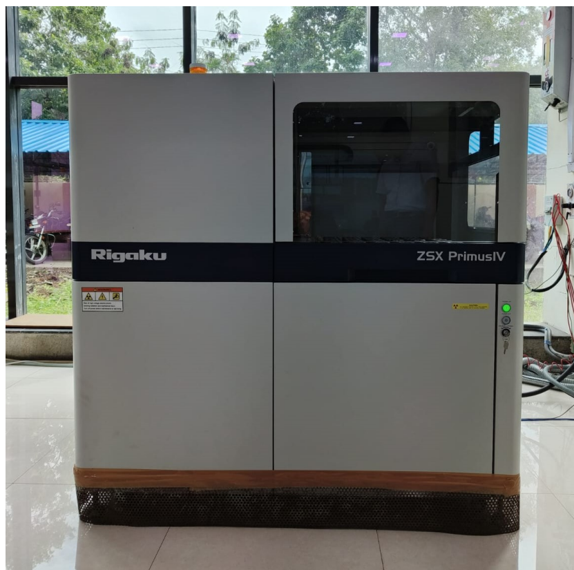
Photo - 11: Photographs showing WD-XRF instrument (Rigaku, Japan) at Chemical Lab, MECL, Nagpur
