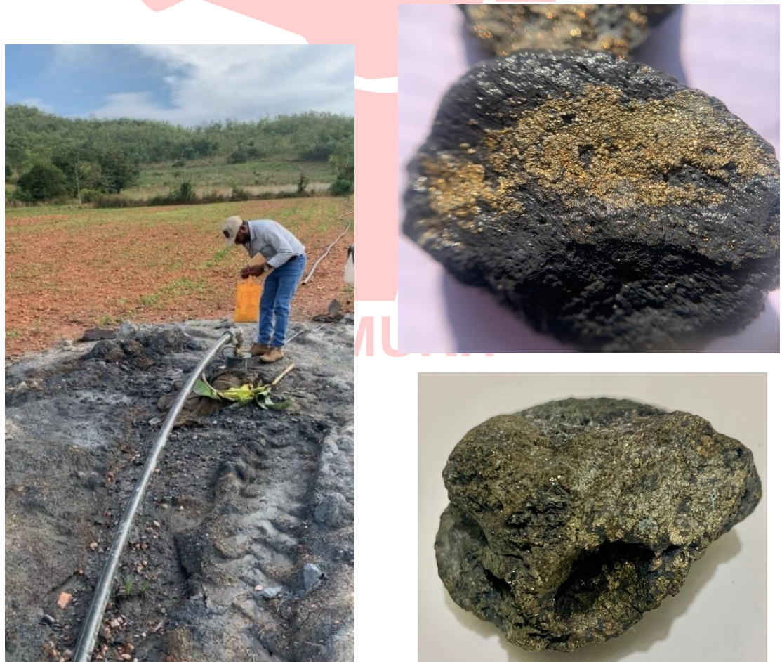
Figure 13: Water well borehole (RC) cuttings containing sulphides (pyrite and chalcopyrite) Sample No : 34 BRS 123
