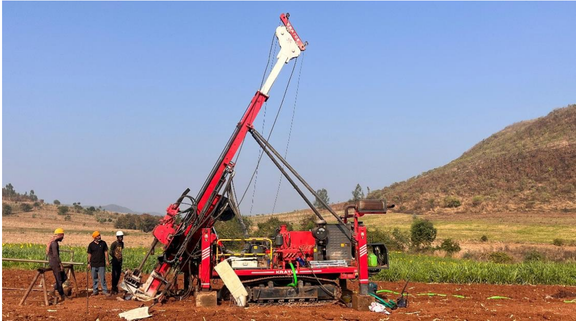
Figure 30 : Kratos 800 hydraulic power rig deployed at site
