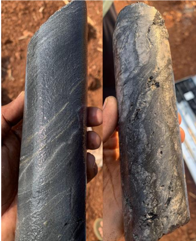
Figure 33: Drill core of BH -01 indicating Carbonaceous Phyllite with veining and pyrite
