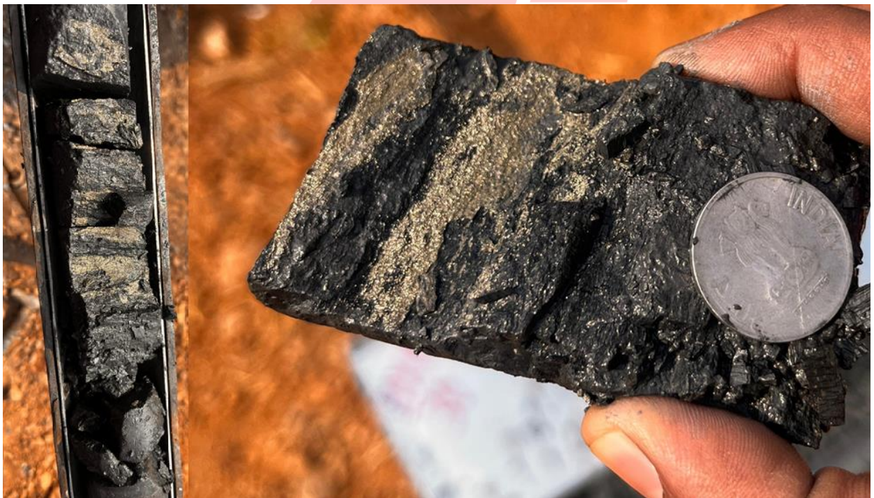
Figure 35 : Drill core cutting of BH 02 indicating Carbonaceous phyllite containing sulphides (Pyrite)
