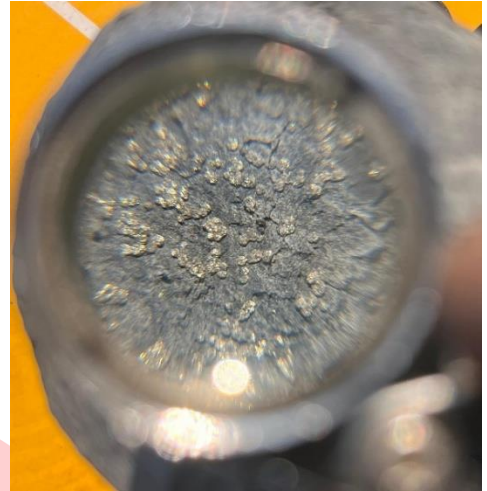
Figure 34 : Pyrite clusters observed in drill cuttings. (BH 01)
