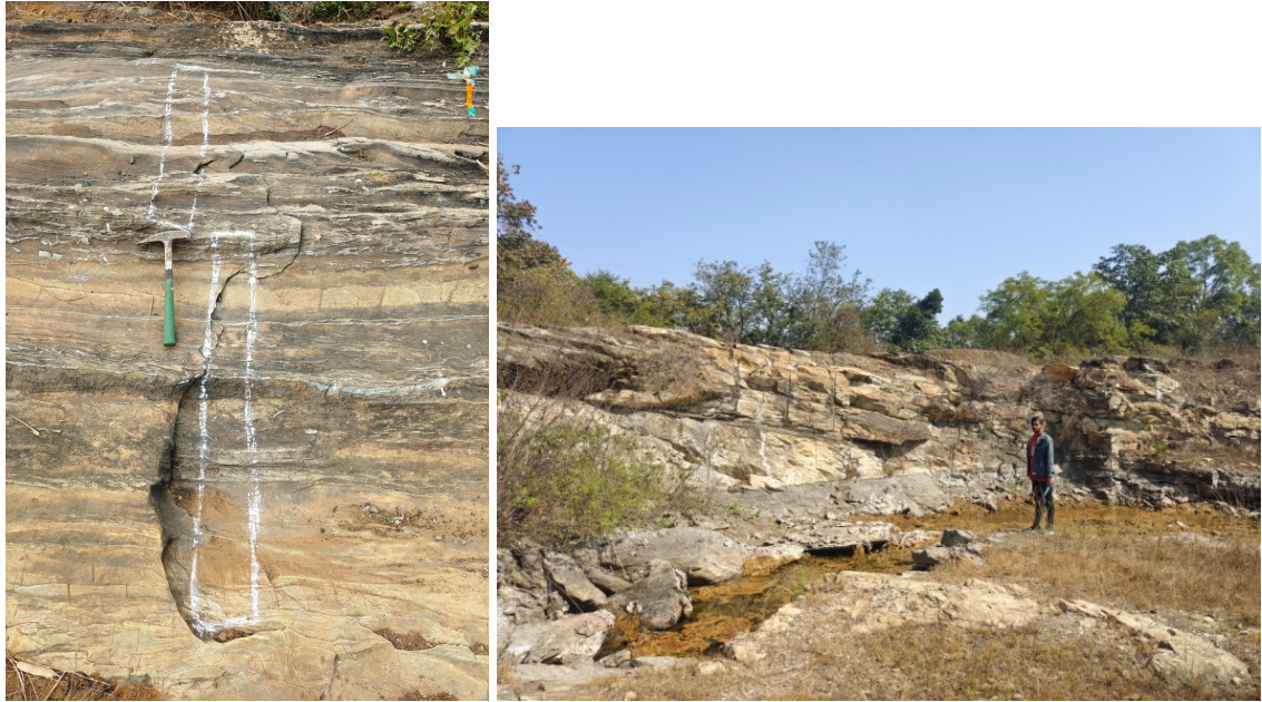
Field Photograph 7.5: Left- Channel marking on the Dolomite for sampleing. Right- Dolomitic shale/Dolomite exposed in the mining pit in the eastern part of Mundatola block.
