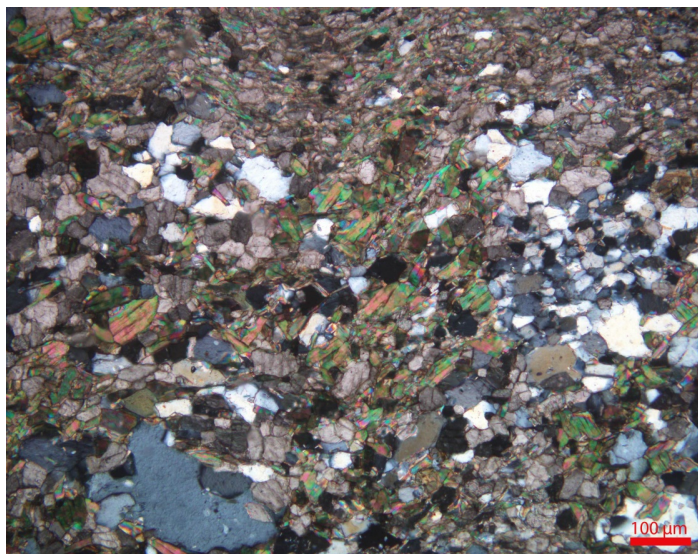
Pmg – 1: Photomicrograph showing association of dolomite, quartz and micaceous minerals in shaly dolostone/ dolomitic shale as seen under crossed nicols. Sample No.: MMLP02 Magnification: 100X
