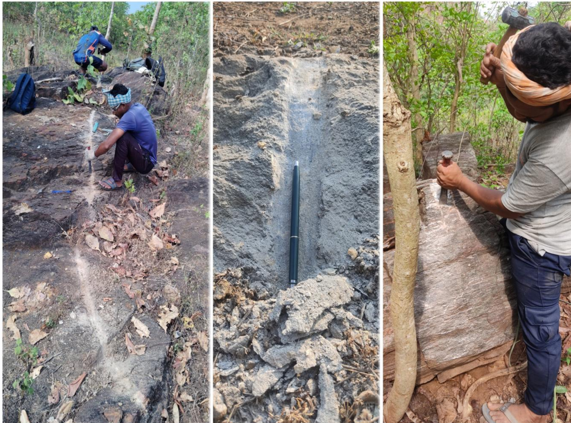
Figure 6.19: Different stages of development of groove in order to collect BRS
