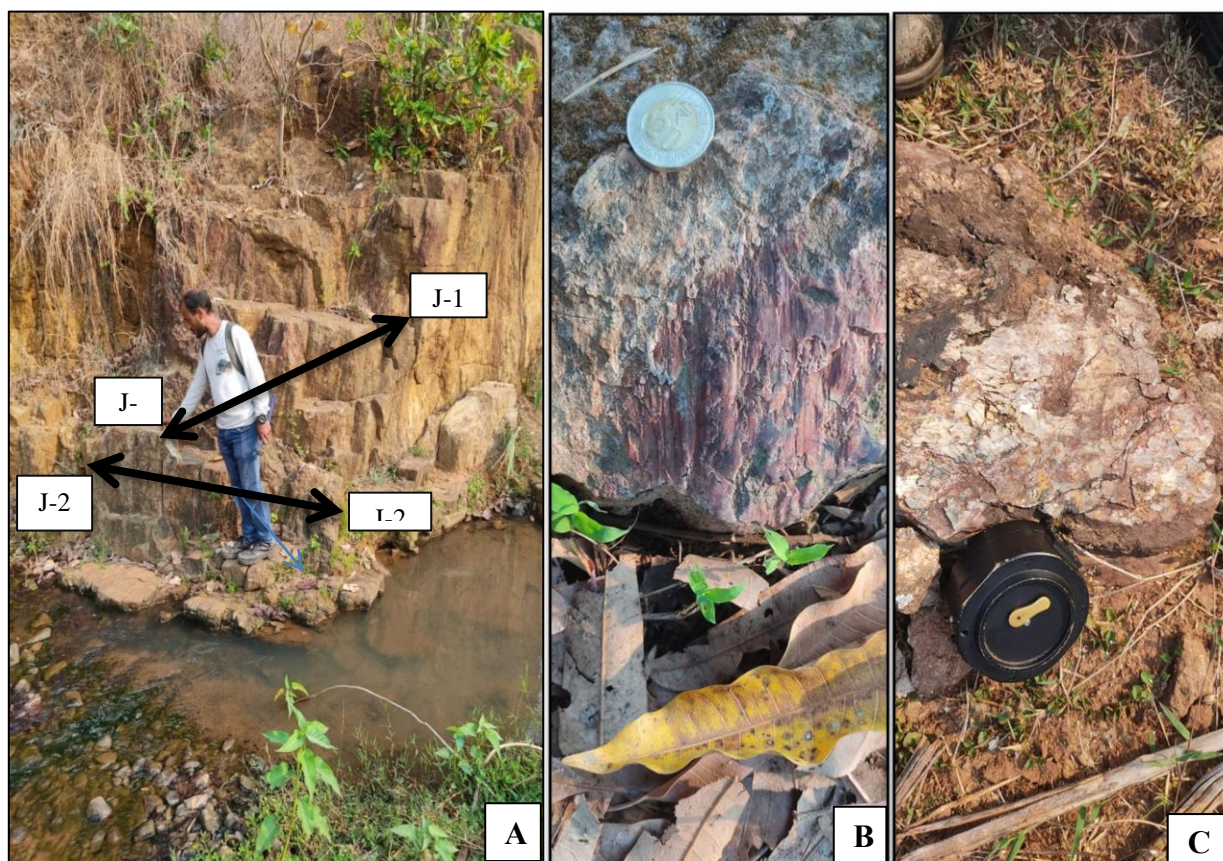
Figure 6.18: Field photographs of A. Joints B. Slickenside preserved on rolled boulder, C. fault gouge preserved on the surface of rolled boulder
