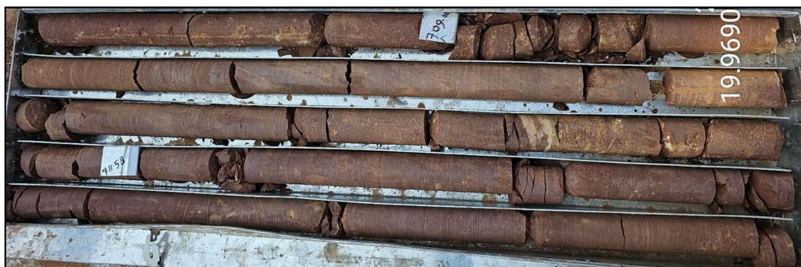
Fig. 2.9.1 Chocolate/reddish brown claystone of Motur Formation as encountered in borehole no. CMWWB01.
