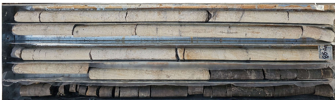
Fig. 2.9.1 C: Seam II B (822.75-826.60m) as encountered in Barakar Formation in borehole no. CMWWB01.
