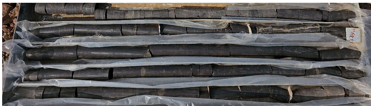
Fig. 2.9.1 A & B : Seams II A (815.60m-818.45m) encountered in Barakar Formation in borehole no. CMWWB01.
