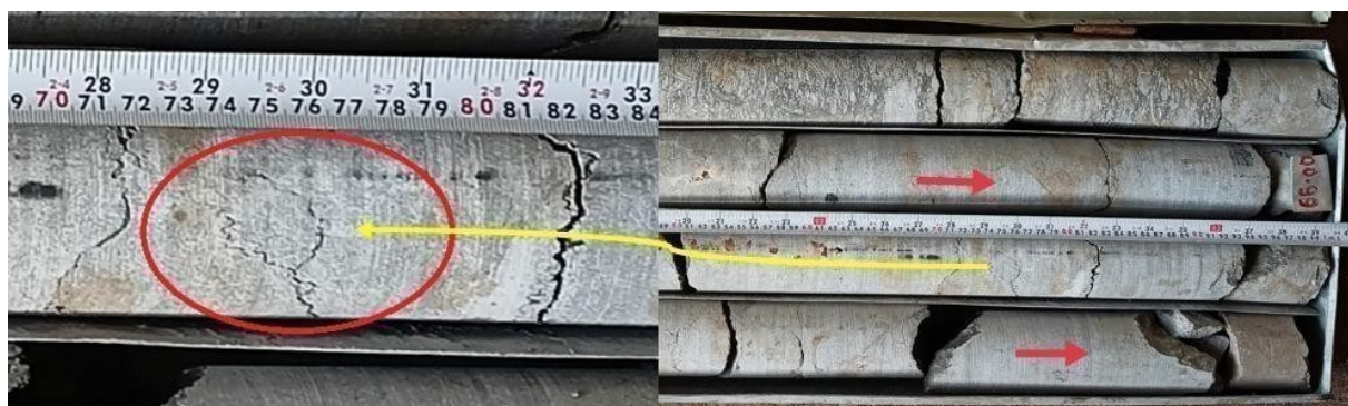
Fig 5.11. Photograph of core of Upper Sylhet Limestone showing Stylolite.
