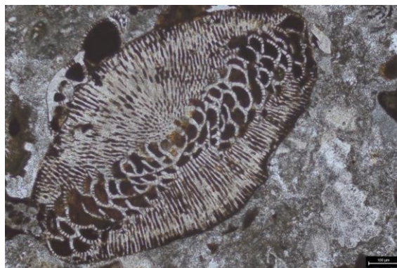
Fig 5.30: Photomicrograph showing Nummulitessp. Foraminifera in PPL
