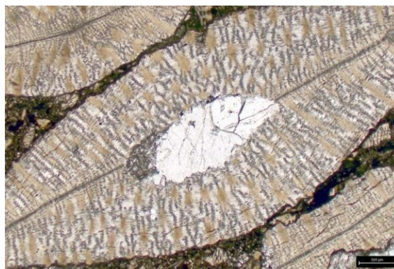
Fig 5.16: Photomicrograph from BLD/C1 showing Discocyclina sp foraminifera in PPL embedded in micritic cement and some fossil cores being altered to calcite grains.
