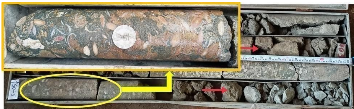
Fig 5.9. Photograph of core of brownish cherry red fossiliferous limestone showing Discocyclina sp and Alveolina sp fossils (PBH-02).
