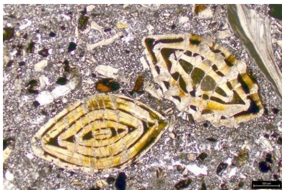
Fig 5.18: Photomicrograph from BLD/C3 showing Nummulites and some Discocyclina sp foraminifera in micritic cement (in PPL)
