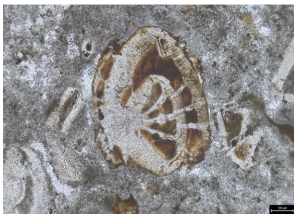
Fig 5.34: Photomicrograph showing bivalve fossil in PPL
