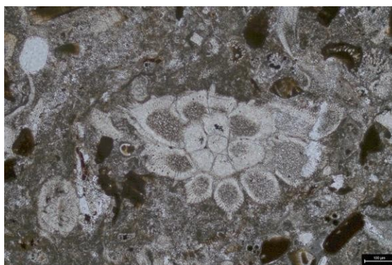
Fig 5.28: Photomicrograph showing Rotalida foraminifera in PPL
