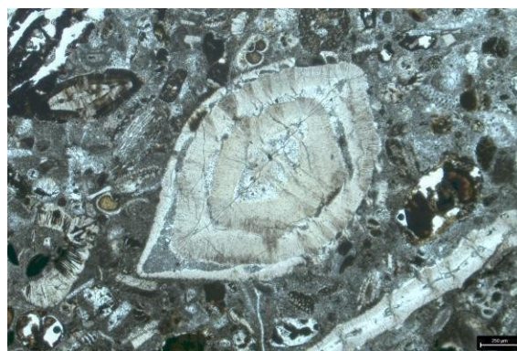
Fig 5.22: Photomicrograph showing Nummulites sp. foraminifera (in PPL)
