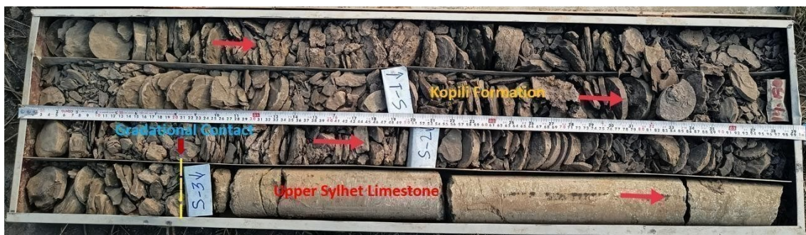
Fig 5.14. Photograph of core showing contact between Kopili Formation and Upper Sylhet Limestone (PBH-03).
