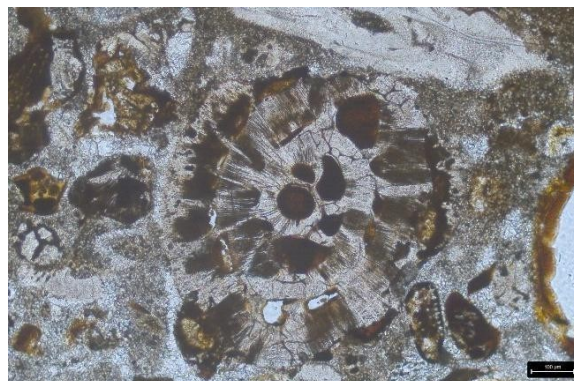
Fig 5.48: Photomicrograph showing Nummulites sp. Foraminifera (in PPL)
