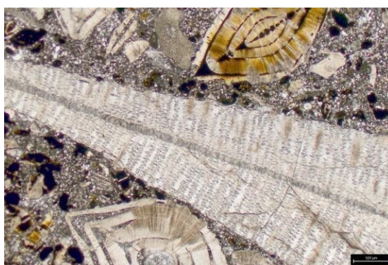
Fig 5.18: Photomicrograph from BLD/C3 showing Nummulites and some Discocyclina sp foraminifera in micritic cement (in PPL)
