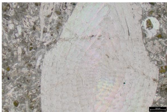
Fig 5.17: Photomicrograph from BLD/C2 showing calcified fossils within spary cement
