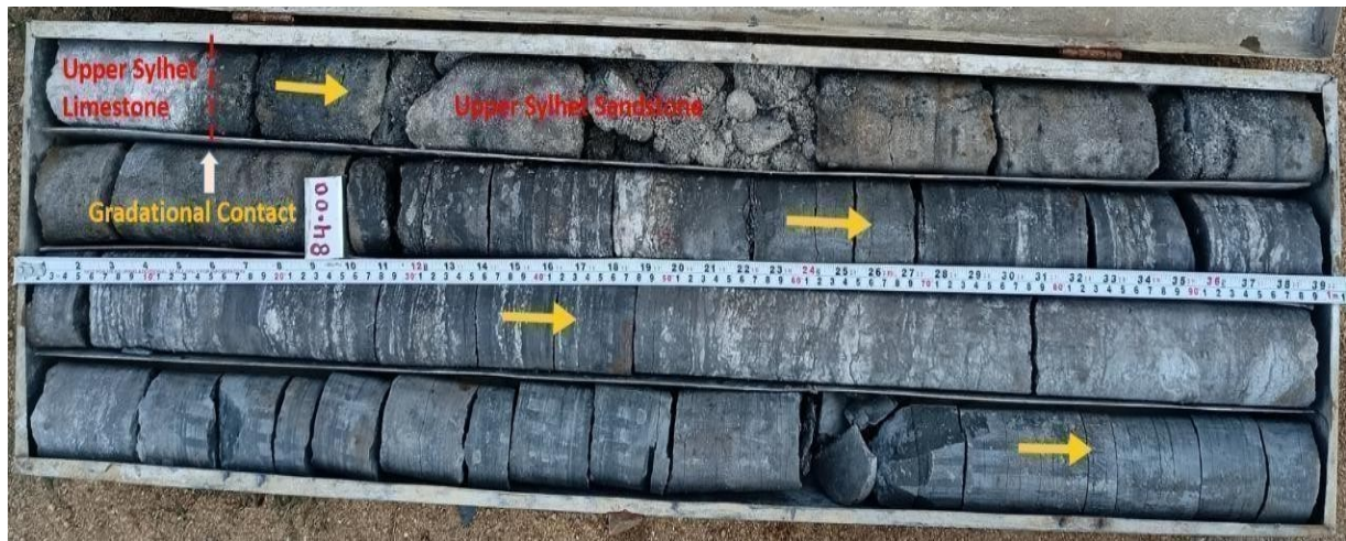
Fig 5.3. Photograph of core showing contact between Upper Sylhet Limestone & Upper Sylhet Sandstone member.
