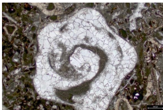
Fig 5.40: Photomicrograph showing Asterocyclina sp. Completely altered by calcite
