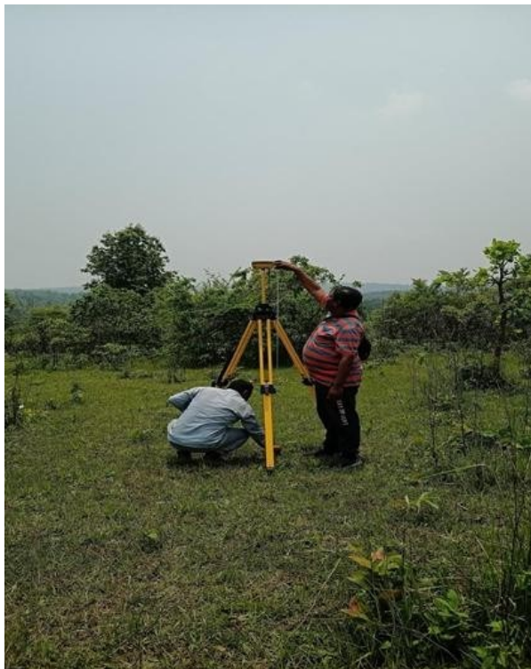
Fig.5.2: Topographical survey done by DGPS
