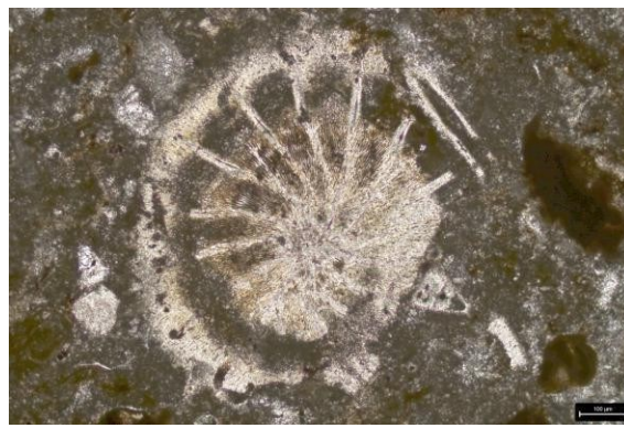
Fig 5.20: Photomicrograph showing bivalve fossil under PPL
