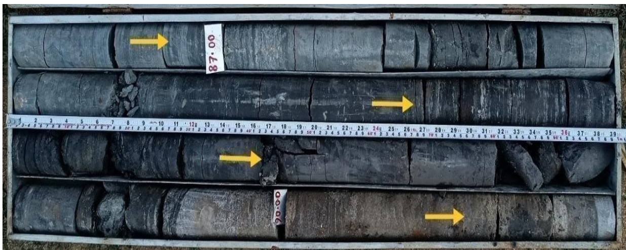
Fig 5.4. Photograph of core showing intercalation of shale and sandstone of Upper Sylhet Sandstone member
