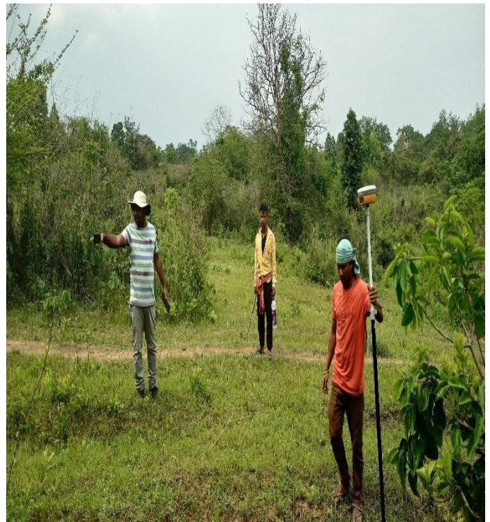
Fig.5.2: Topographical survey done by DGPS
