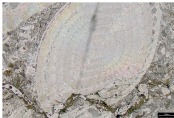
Fig 5.17: Photomicrograph from BLD/C2 showing calcified fossils within spary cement
