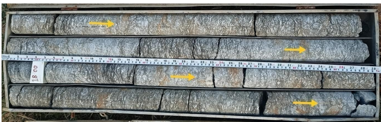
Fig 5.10. Photograph of core of highly fossiliferous limestone of Upper Sylhet Limestone encountered in borehole PBH-01 (15.92m to 19.93m depth)
