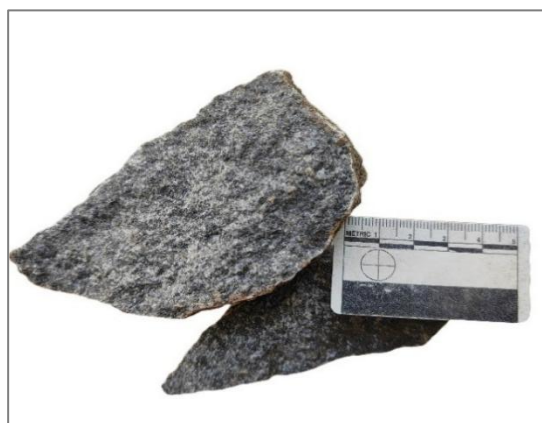
Field Photograph 17: In hand specimen, these are melanocratic, medium-grained, mafic igneous rock and magnetic in nature.
