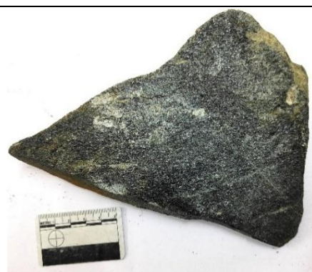
Field Photograph 13: In hand specimen, Metagabbro appears as melanocratic, medium to coarse grained. The greenish tinge may be due to Chloritization.
