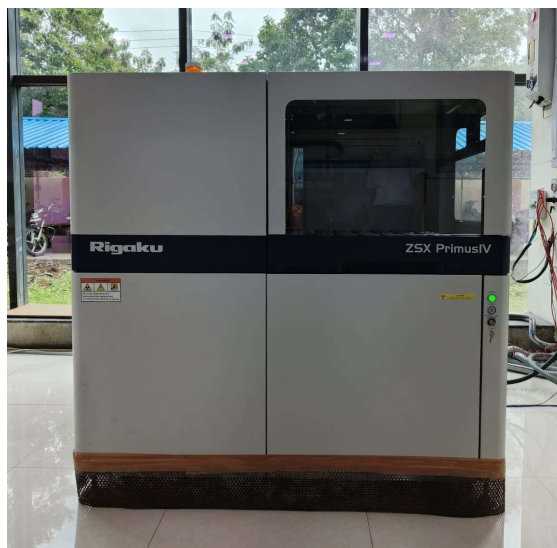
Photo 8 - Photograph showing WD-XRF instrument (Rigaku, Japan) at Chemical Lab, MECL, Nagpur
