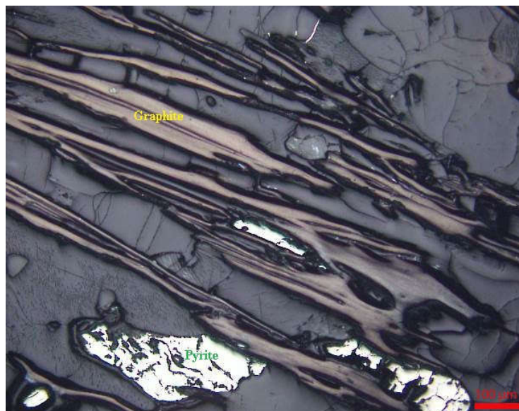
Pmg – 3: Photomicrograph showing fine to medium plates and flaky aggregates aligned along the foliation and associating fine to medium anhedral grains of pyrite as seen under reflected light. Specimen No.: MBMGM-01 (MBMG-08/70.40-70.50m) Magnification: 100X
