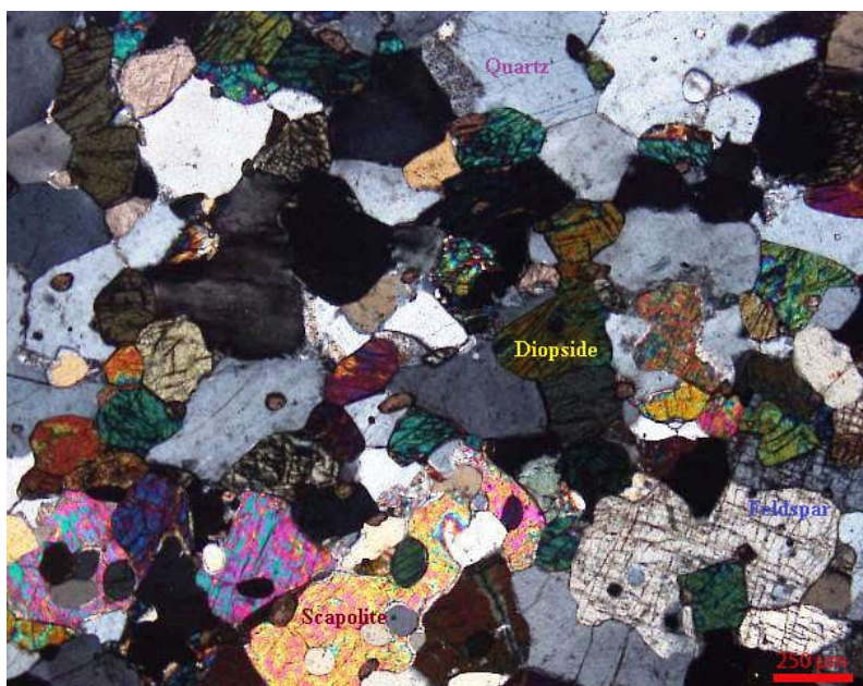
Pmg – 2: Photomicrograph showing association of quartz, diopside, scapolite and feldspar in meta-calc silicate as seen under crossed nicols. Specimen No.: MBMGP-02 (MBMG-02/14.20m – 14.30m) Magnification: 40X
