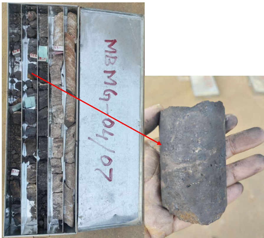
Field Photograph 10.3: Photograph showing drill cores of (Khondalite associated with manganese mineralization) Borehole No. MBMG-4 and close view of the core at 35.25m
