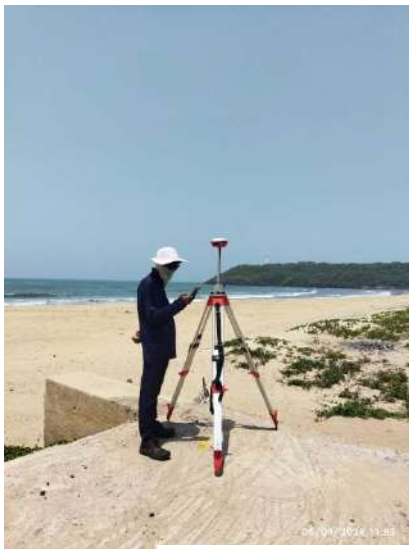
Carrying out the Level transferring near Achara light house
