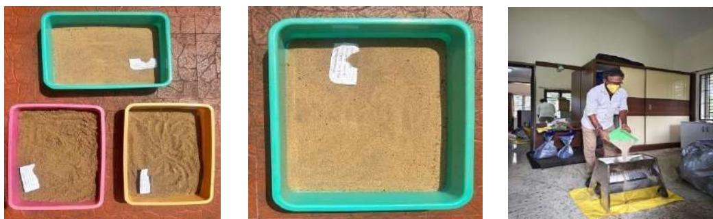
Plate.8.1 Sample processing procedures (a & b) Sun-drying (c) Coning and Quartering
