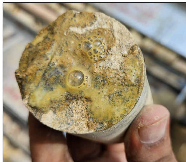
Fig. 7.12: Yellow effervescence on reaction of Shapiro solution in contact of phosphorite.
