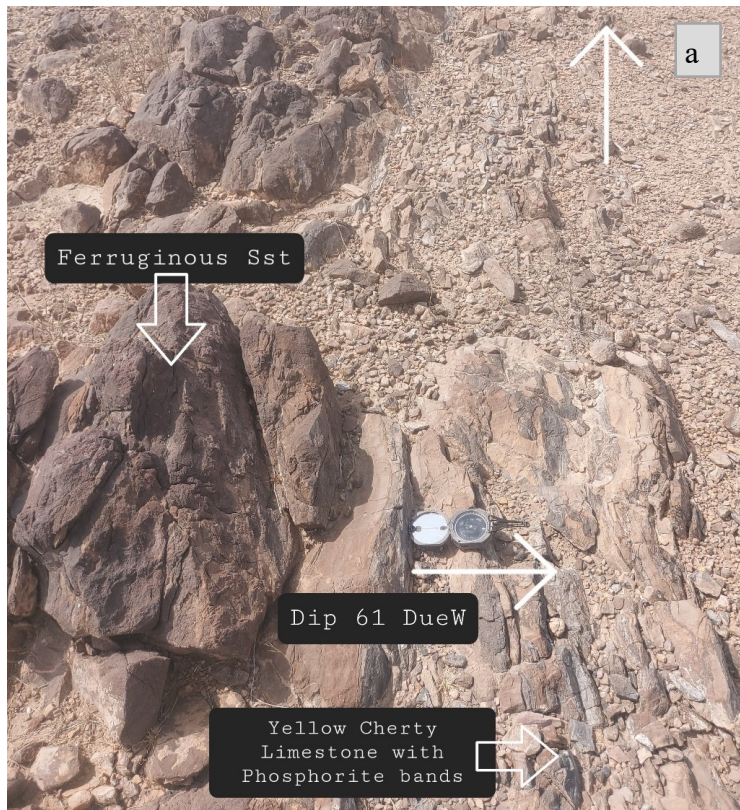
Fig 7.5 (a) Ferruginous Sandstone in contact with phosphatic limestone exposed along section line S3-S3'
