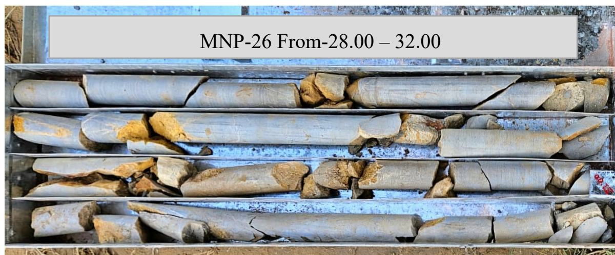
Fig. 7.15 Dolomitic limestone intercepted in borehole no MNP-26 28.00 to 32.00m.
