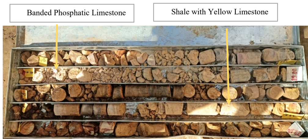
Fig. 7.11. Banded phosphatic limestone in BH MNP15 from 17.00 to 22.00m.
