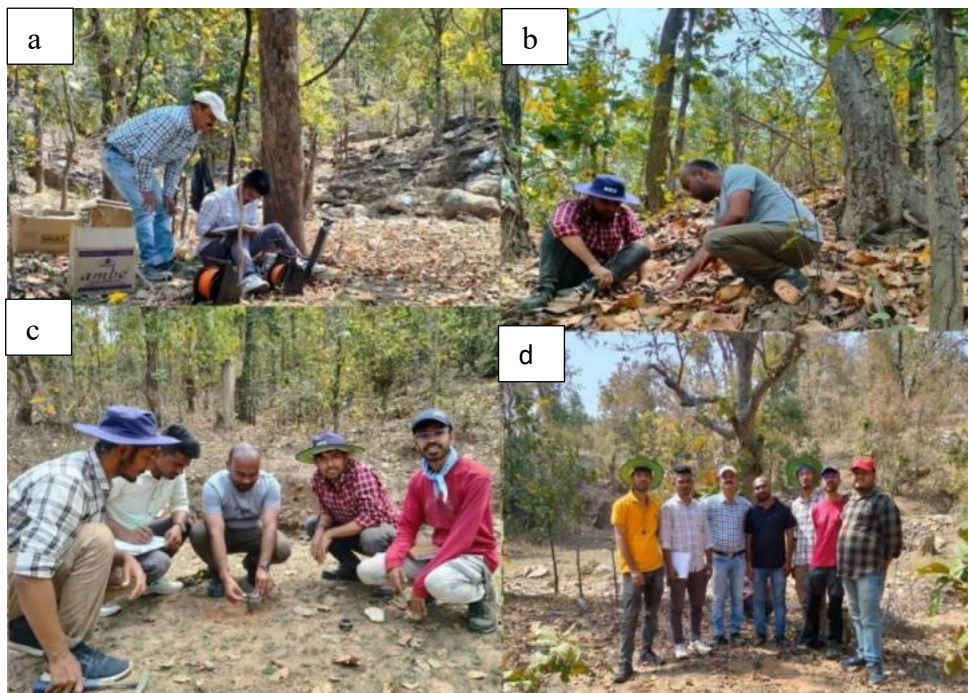
Fig no-16 : (a) SP data recording in DDR3 instrument, (b), (c) Base electrode and rover electrode establishment, (d) team of the geologist and geophysicist involved for this survey.
