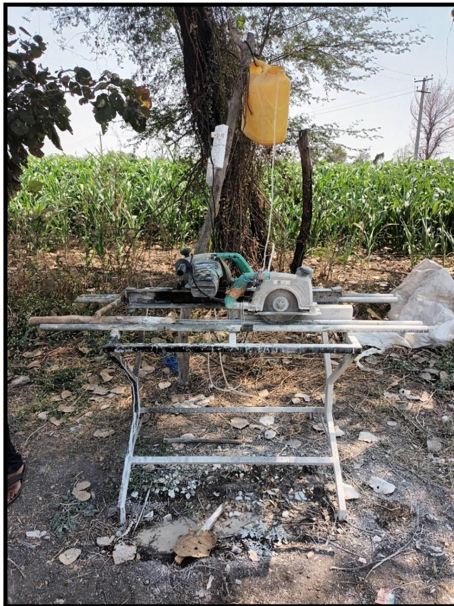
Photograph -2 : Photograph showing Core cutting machine in operation at field.
