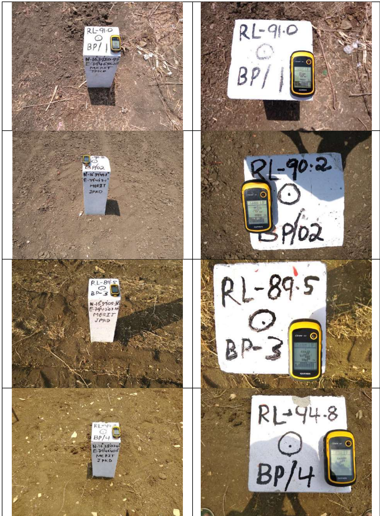
Figure 2.3 A. Photographs of boundary pillars BP 1 to BP 4 with GPS reading in Madinapadu limestone block
