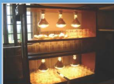
Drying of samples using IR lamps
