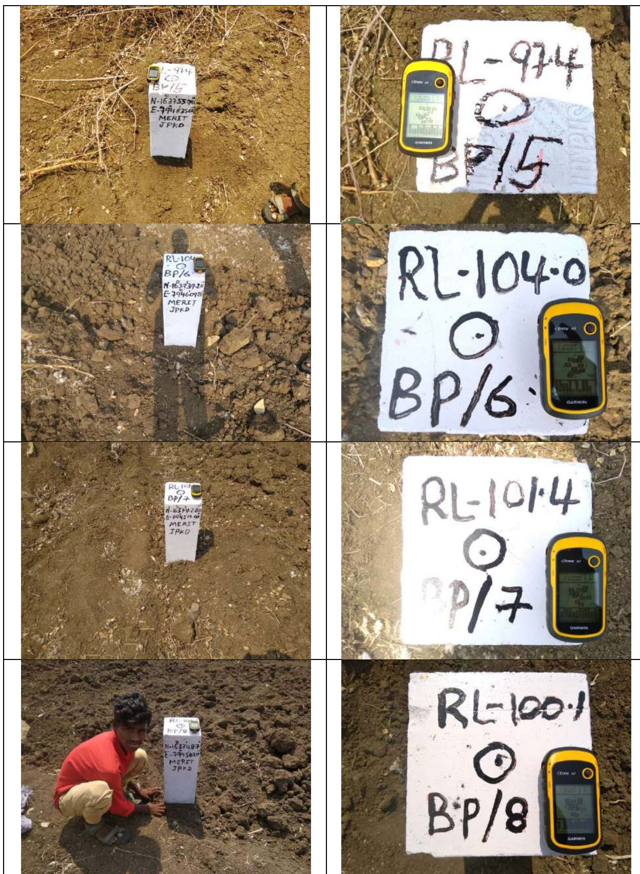
Figure 2.3 B. Photographs of boundary pillars BP 5 to BP 8 with GPS reading in Madinapadu limestone block
