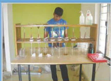
Bromoform separation of Heavy minerals
