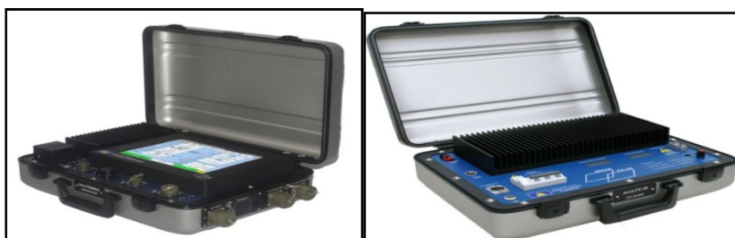
Fig: 2.3.2 Terra TX and TEM used for TDEM survey
