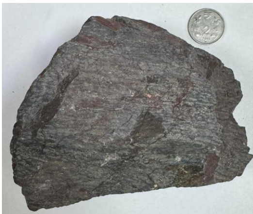
Figure 4.9. Hand specimen of the representative pyroclastic rock sample (Sample No. IBM/SRC/REE/GR/(412/05)/PC/PS/04) collected from the Siwana Ring Complex, Rajasthan, showing its dark grey to reddish-brown color, compact nature, and fine-grained pyroclastic texture with lithic fragments embedded within a fine-grained matrix.
