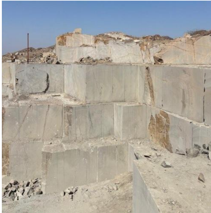
Figure 3.5. Active granite quarry in the Siwana Ring Complex exhibiting massive, blockable granite for dimension stone extraction.
