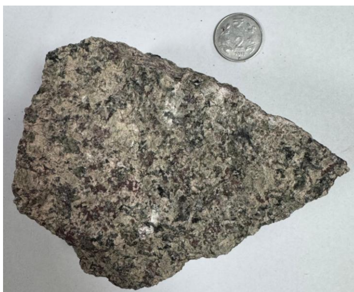
Figure 4.5. Hand specimen of the representative granite sample (Sample No. IBM/SRC/REE/GR/(232/02)/GR/PS/12) showing its light grey colour, leucocratic nature, and porphyritic texture with conspicuous feldspar phenocrysts.
