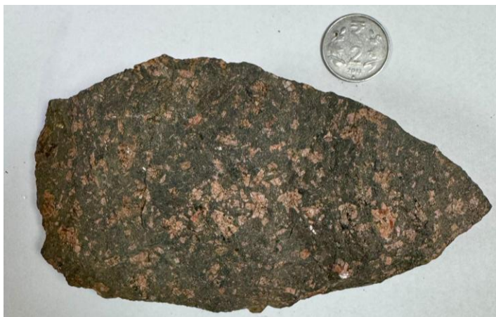
Figure 4.7. Hand specimen of the representative trachyte sample (Sample No. IBM/SRC/REE/GR/(78/22)/TR/PS/07) showing its dark grey colour, porphyritic texture, and pinkish alkali feldspar phenocrysts embedded within a fine-grained groundmass.
