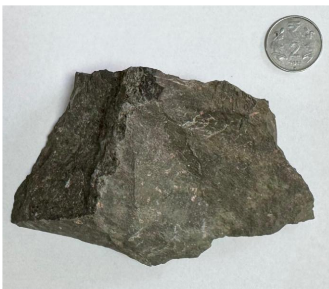
Figure 4.3. Hand specimen of the rhyolite sample (Sample No. IBM/SRC/REE/GR/(131/06)/RH/PS/05) showing its dark grey colour, massive nature, and fine- to medium-grained texture.
