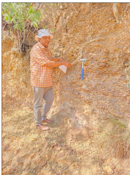
Photo No – 6: The exposure is located about 3.34 km east of Lakhond village and approximately 2.01 km from the SH-42 road. Laterite/bauxitic clay of pinkish to yellowish-white colour, with lenses of yellow clay, is exposed along the right bank of nala. The exposure extends for about 30 m in length and approximately 2 m in height, and contains occasional lenses of white clay and iron oxide patches.
