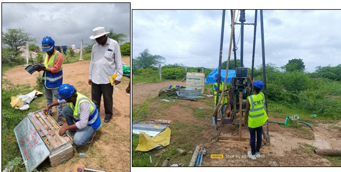
Photo No: 40 Calyx rotary drilling machine used for drilling in Lakhond Area, Kachchh District, Gujarat
