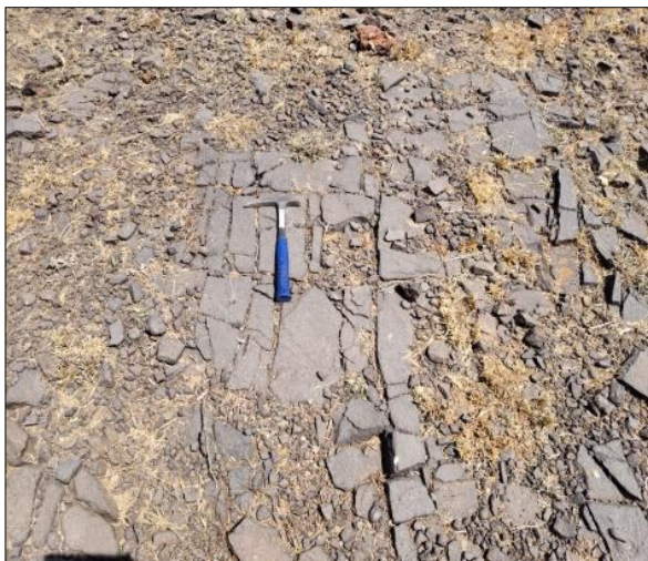
Photo No – 5: The area is situated approximately 1.47 km to the northeast of Lakhond, on the west side of the water tank, along the pediment area composed of reddish-brown, fine- to medium-grained, splintery ferruginous sandstone on the surface showing 2 sets of joints.
