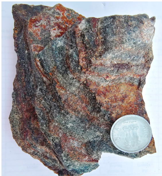
Photo-5 Magnetite quartzite outcrop with sulphides, NW of Vartanapalli
