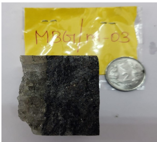
Photo:19: Borehole core photograph showing Amphibolite with pyrite disseminations (MBG-02/MBG/M-3 @ 94.10-94.20m)
