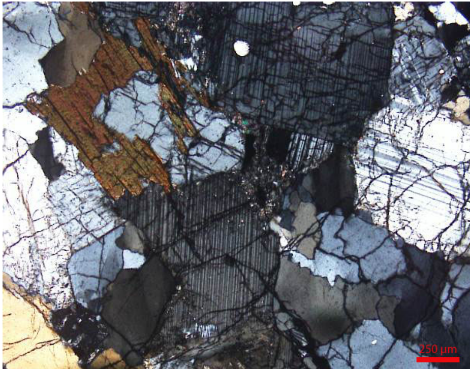
Pmg – 2: Photomicrograph showing association of plagioclase, quartz and biotite in granodiorite as seen under crossed nicols.
