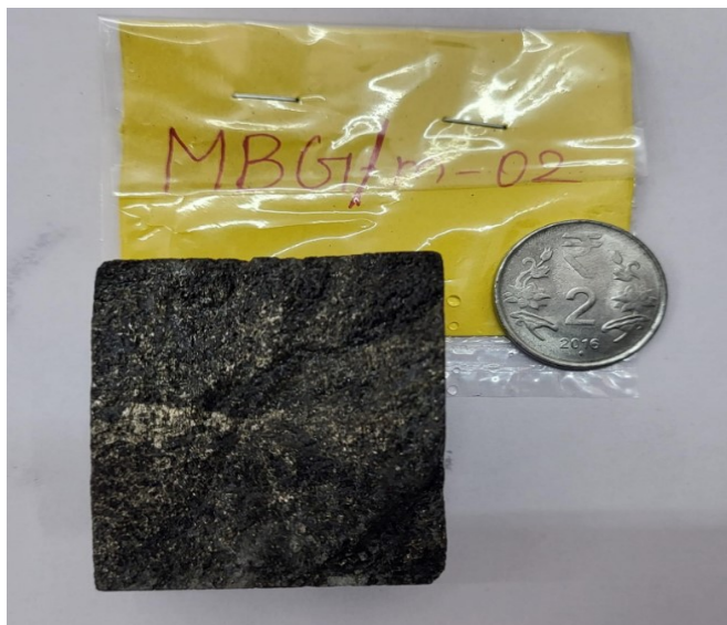
Photo:18: Borehole core photograph showing Amphibolite mostly with pyrrhotite and specks of pyrite (MBG-01/MBG/M-2: @104.80-104.90m)
