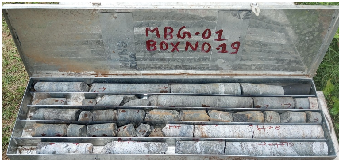
Photo-16: Borehole core photograph showing schistose Amphibolite with carbonate veins followed by silicified Amphibolite (MBG-01: Depth 95.0m – 100m)
