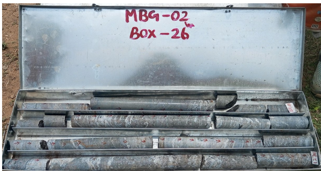
Photo:17: Borehole core photograph showing Gt.bearing schistose Amphibolite with thin quartz veins with pyrite dessiminations. (MBG-02: Depth.123.00-124.70m)
