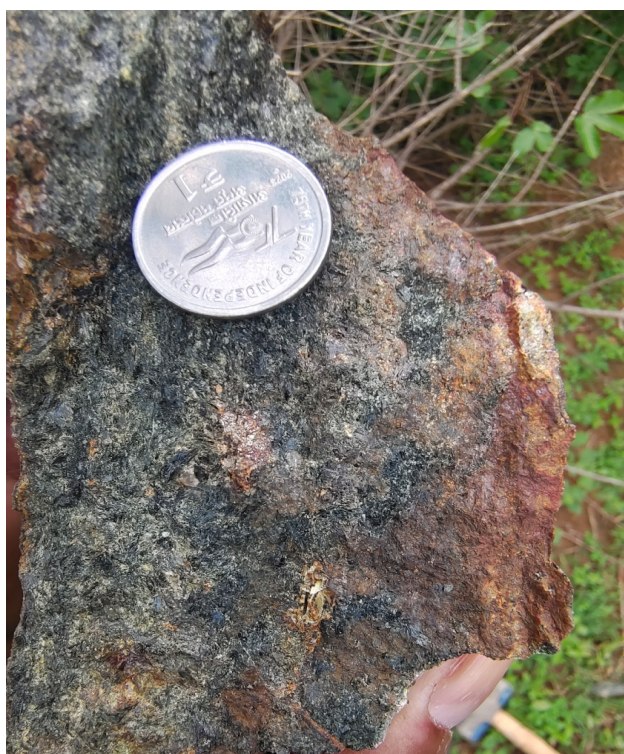
Photo-3 Sheared Amphibolite with alteration and sulphides
