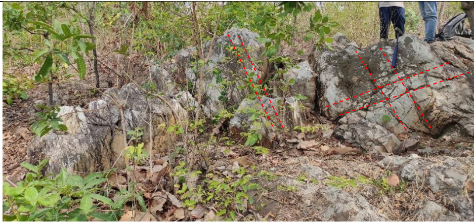
Field photograph: Two joints set, J1 trending N64E and J2 trending N45W, are common in the area of investigation, north of Jharegaon village (21.91518,77.83473).
