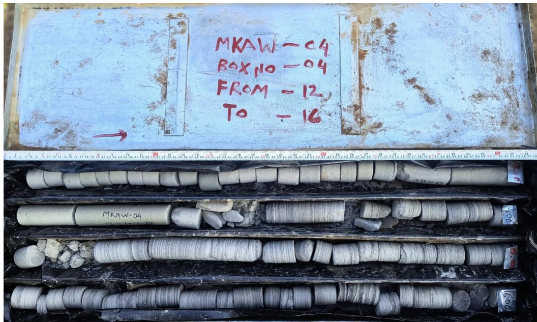
Photograph showing glauconite & Alternate band of glauconite horizons (Sandstone and Shale) in Borehole no- MKAW-04 (Depth-12.00m to 16.00m).
