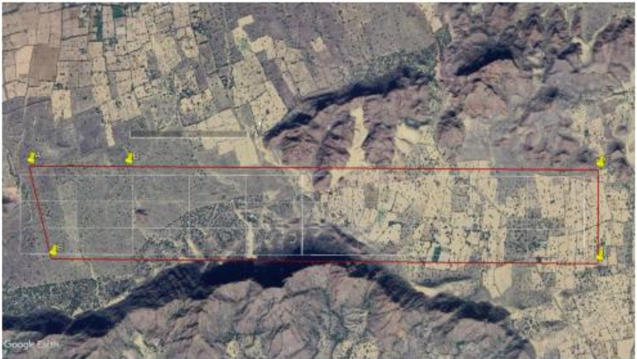
Fig. 5: Plan of proposed 40 vertical boreholes in G3 stage exploration in the khera khindawara block on a 400m*200m grid.
