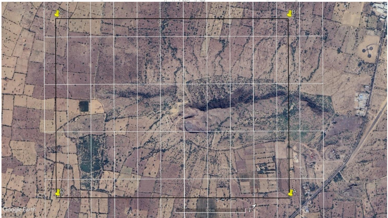
Fig 4: Plan of proposed 40 vertical boreholes in G3 stage exploration in the North of Muthli block for FS 2026-27. The spacing of boreholes will be tentatively 400m*200m.
