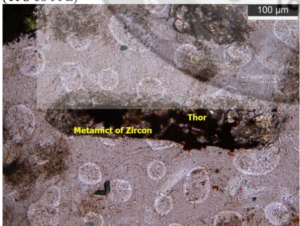
Fig 7.5: Metamict of zircon with thorite in granite TPS-20 (PPL)
