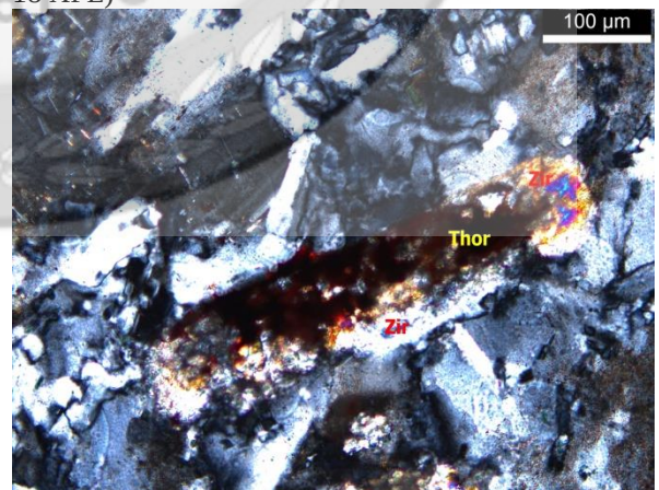
Fig 7.6: Metamict of zircon with thorite in granite TPS-20 (XPL)
