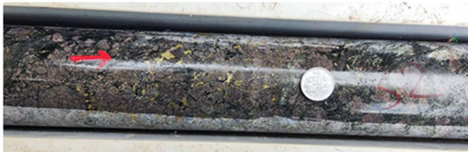
Photo 18: Stringers, veinlets and sheeted interconnected veins of Chalcopyrite and Pyrite mainly occurring along porphyroblastic garnetiferous mica schist (MTB-4)
