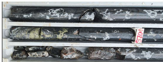
Photo 19: Massive thick fracture filling vein of Cpy, at contact of Granitic rock with Meta-basics. (MTB-5)
