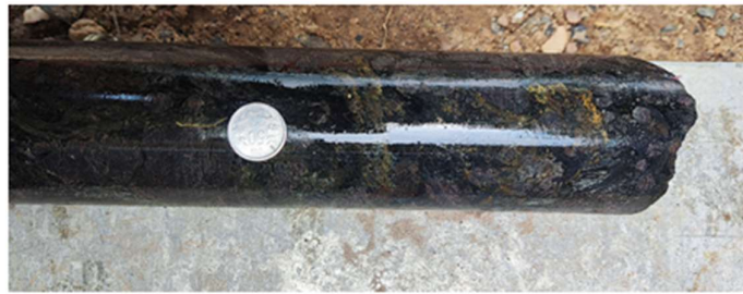
Photo 17: Stringers, veinlets and sheeted interconnected veins of Chalcopyrite and Pyrite, mainly occurring along porphyroblastic garnetiferous mica schist (MTB-4)
