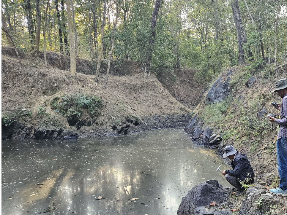
Figure 3: Waterlogged old excavated pit in the area, Mn reefs seen alongside the excavated pit wall. Regional trend for pit is E-W. (Location: 377931, 2383157)
