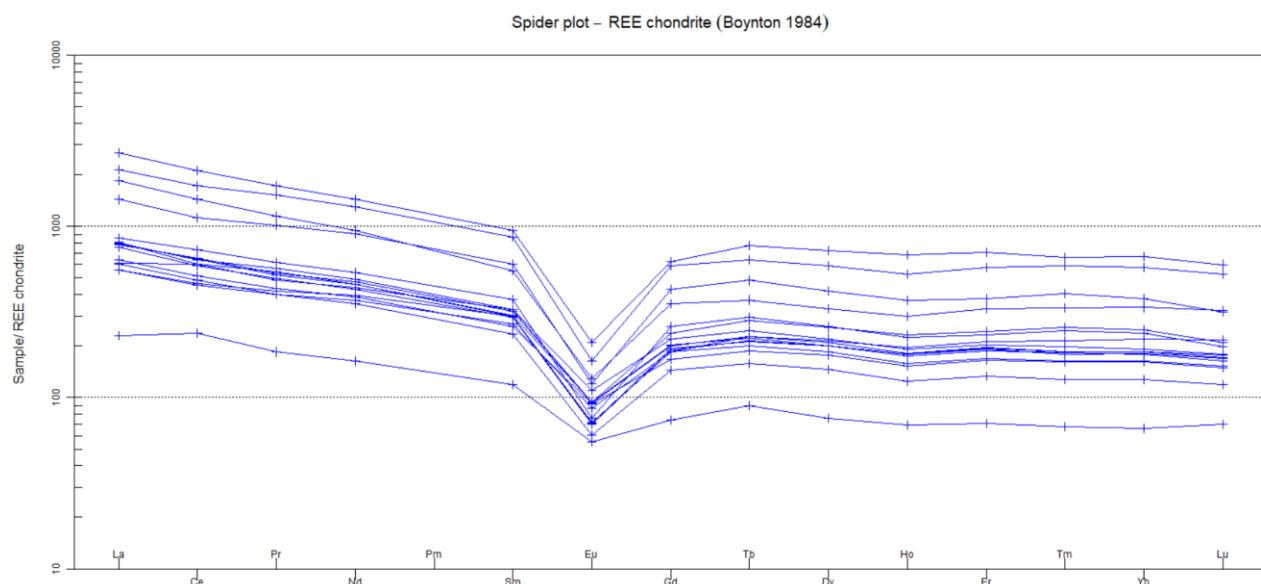
5.5.0 The Chondrite normalized spider plot (Boynton 1984) for samples analysed from rhyolites reveals the flat trend of REE with slightly enriched LREE. The strong negative Eu anomaly has been observed in the diagram.
