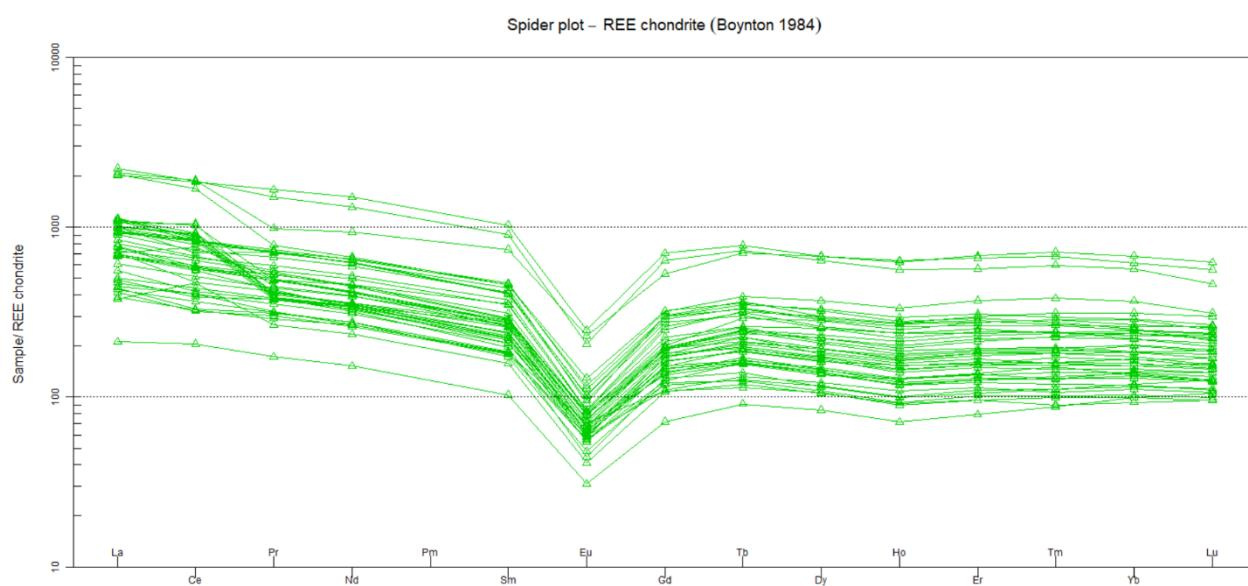
5.3.0 The Chondrite normalized spider plot (Boynton 1984) reveals the flat trend of REE with slightly enriched LREE. The strong negative Eu anomaly has been observed in the diagram.
